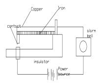
The diagram shows an automatic fire alarm. When there is fire the heat cause the copper to expand more than the iron over the same temperature rise. When the temperature of the place where it is fixed reach a certain predetermined value the bimetallic strip curve inward and the contact point closes. This set the current flowing and causes the alarm bell to ring.
