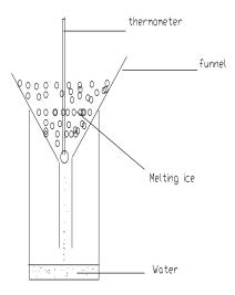
Insert the thermometer inside a mixture of ice and water (melting ice) as shown above. After the mercury level in the capillary (stem) has remain steady for some time. Note whether this corresponds to the  $0^{0}$ C mark on the thermometer. If not then, the lower fixed point is not accurate.
