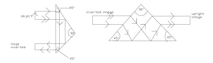
This prism is a right angled isosceles triangular prism. They are used in Periscope, prismatic binoculars, cameras and projection lanterns. The critical angle for glass is about  $41^{0}48^{1}$ . when light enters the prisms as shown it strikes the hypotenuse face at an angle greater than the critical angle and therefore suffer total internal reflection inside the prism following the path shown to get out of the prism.
