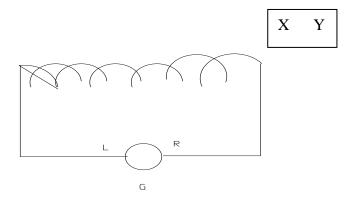
Lenz's law of Electromagnetic induction states that the induced current is in such a direction as to oppose the change producing it by its magnetic action. If the pole of magnet marked X is north-pole, then when it is moved towards the coil the galvanometer should deflect to the right hand side and if this pole is South Pole then it will move to the left when the magnet is moved towards it. In this way the pole of the magnet can be determined exactly.
