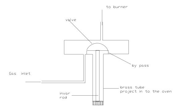
The diagram above shows the Gas thermostat. The brass tube projects into the oven. As the oven temperature rises, the brass tube expands causing the invar rod, which hardly expands to move downwards. The invar in turn moves the valve down reducing the gap between the By-Pass and it, thus reducing the gas flow. At a predetermined temperature the valve will completely be pulled down tightly on the by-pass thus shuting of the gas supply completely
