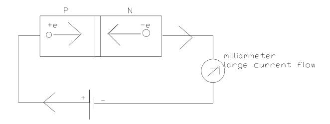
When forward biased large current can flow, the positive hole and the negative electrons are being forced together across the junction and since unlike charges have attraction for each other, the resistance to current flow is low in this case. The current voltage characteristics is shown in figure
