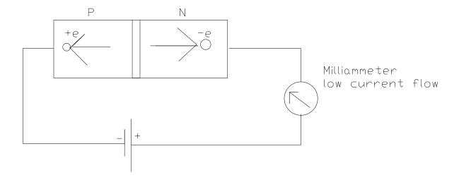
In the reverse biased condition electrons and holes are being forced apart. This require more energy and current does not flow easily. In this case the junction exhibits high resistance.
