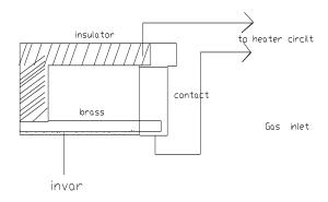
The diagram above is used to control the temperature of an electric heating device. Electric current can flow as long as the contact remains touching. When the temperature around the bimetal strip made of invar and brass reach a predetermined value, it bends away from the contact as brass expands more than invar (which have very low thermal coefficient of expansion). The contacts are broken and current seizes. On cooling, the contact is again remade and the heater is switched on.
